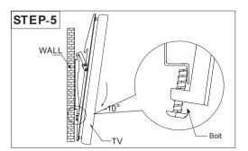
Step 5: Tighten the screw of the two hanging arms to make sure the TV has been fixed firmly.
