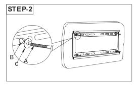
Step 2: Install the wall plate. Put the wall plate on the wall, and then screw four self-tap screws into each plastic anchor through metal washer to fix the wall plate onto the wall.
