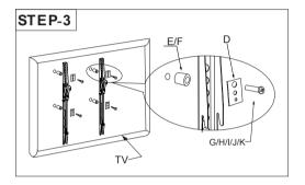
Step 3: Install the bracket rail onto the back of the TV: Select suitable screws from the screw package according to the size of the holes in the back of TV. Fix the two hanging arms onto the back of TV by screws into the holes.Make sure equal height of the two hanging arms.
